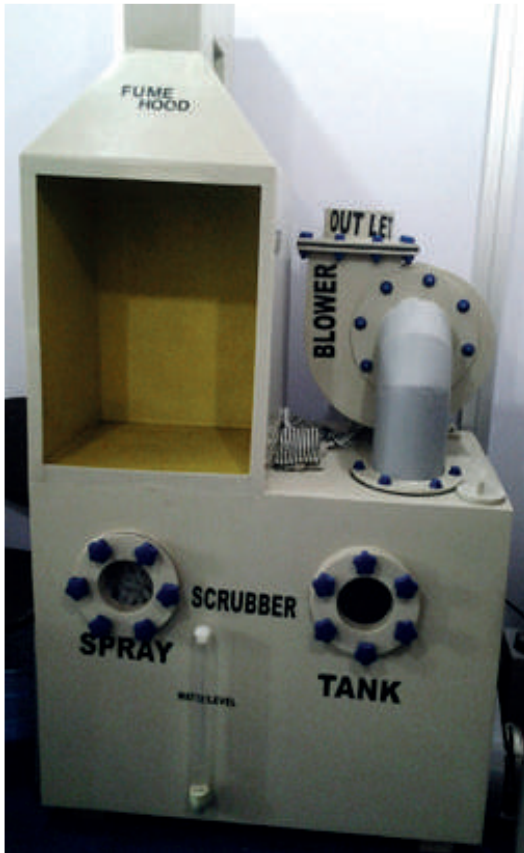
FUME HOOD WITH SCRUBBER
